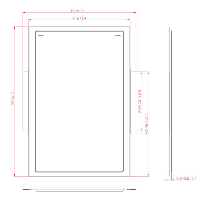
Figure 1 Lithium ion Rechargeable Cell Outline Drawing
